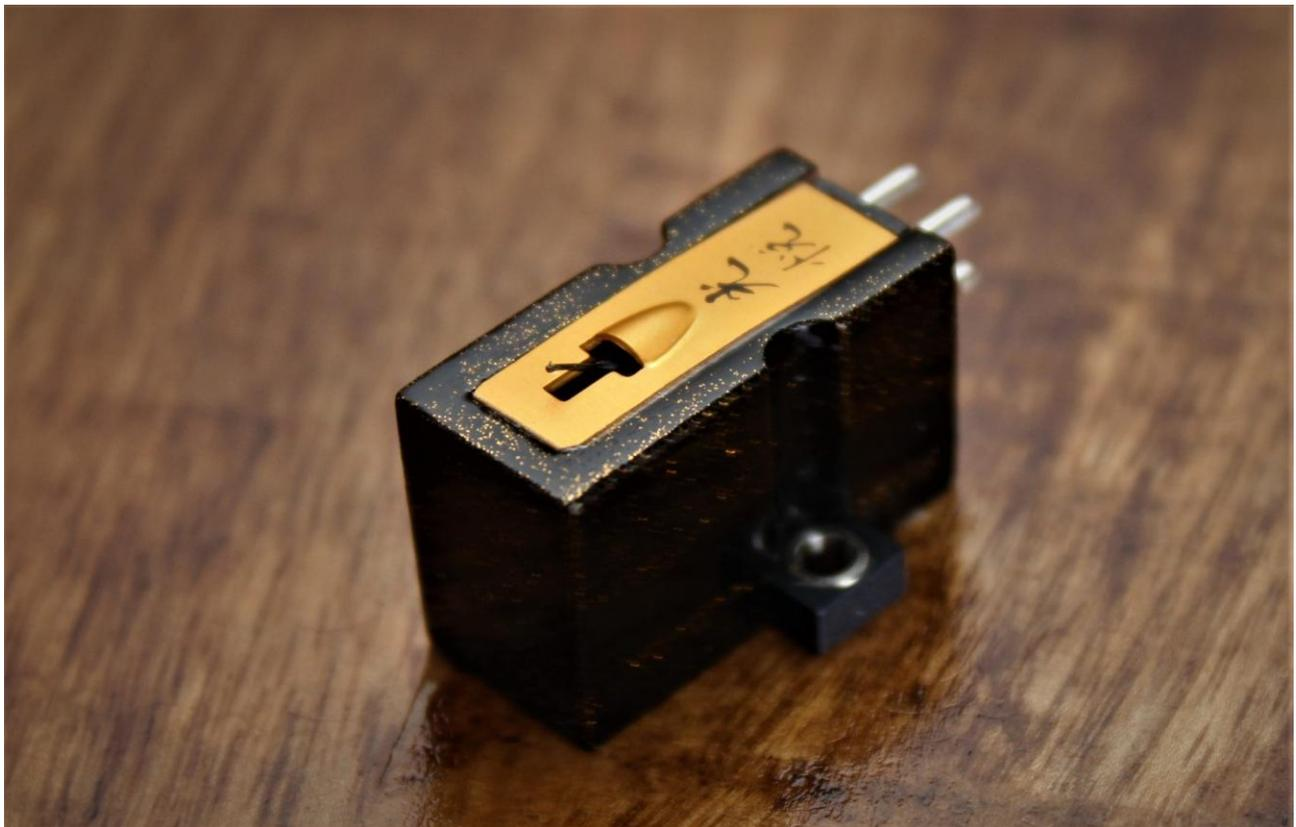
Even though I'm not the biggest proponent of step-up transformers, I do realize that Koetsus prefer them. The only other time I've needed an SUT was to fix an impedance mismatch between a Yamamoto Sound Craft phono stage and that Rosewood Standard. Yamamoto-san made me a custom stereo pair of SUTs and the noise issue was fixed.
